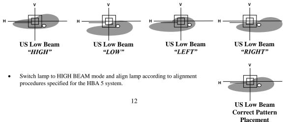
Switch lamp to LOW BEAM mode and visually observe placement of low beam on rear alignment screen of HBA 5. Pattern should be in a relative position of alignment and appear as pictorial.
