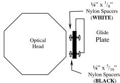
Place a thick nylon bushing on the screw and insert screw through the holes provided at the top of the mast, place a thick nylon bushing on screw and selflocking nut.
