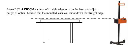
Adjust the rear floor slope wheel until the level in the optical head is centered. Readjustment of height of optical block may be necessary.
