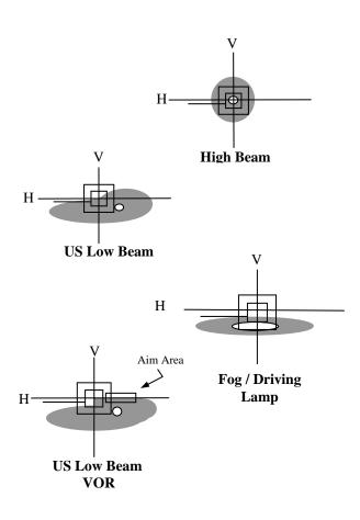
vehicles. The high intensity area is located in the lower right hand quadrant and the beam pattern is aligned by placing the left upper portion of the beam pattern on the .4 Degree (2.096") Down Horizontal axis.
