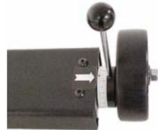
**NOTE:** When rotating eccentric axle on **BCA 4 ISOColor**, both measurements will change at front and rear vehicle wheels, to achieve equal measurements, more than one eccentric axle adjustment may be required.
